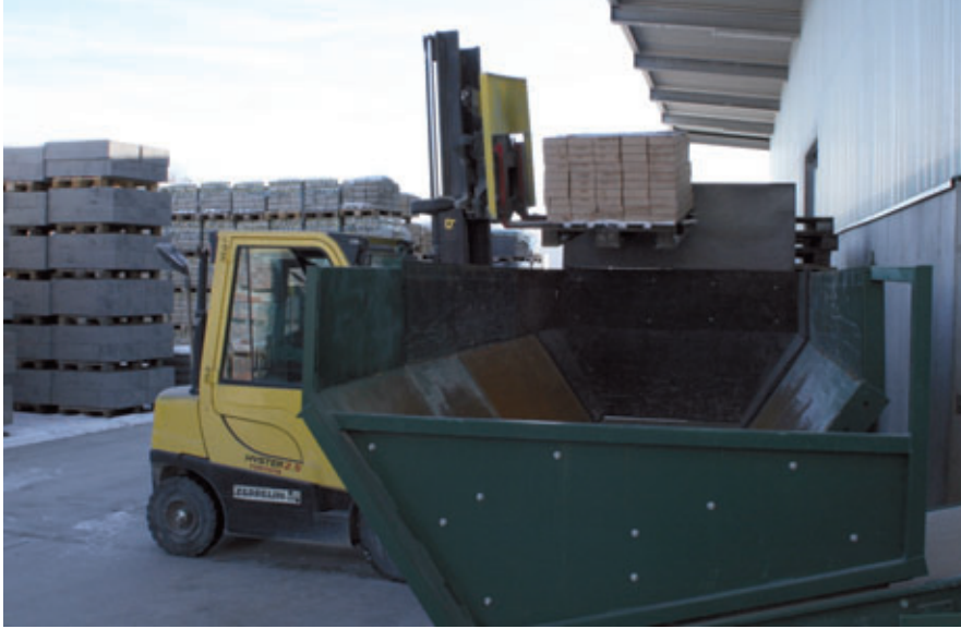
At the outset of the ageing process, the concrete blocks are fed into an accumulation bin by the pallet. From there, they are placed in batches on a conveyor belt to be transported to the ageing drum
