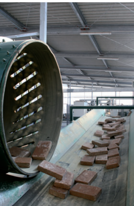
Once they have passed through the ageing drum, the tumbled blocks arrive at a conveyor belt that transports them to the Organizer
