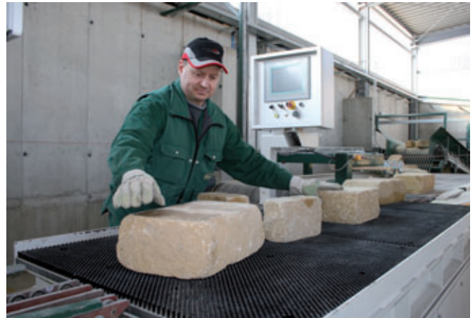
The heavy blocks seem apparently to float on the Magic Table. An employee can sort and feed them to the packaging unit quite effortlessly
