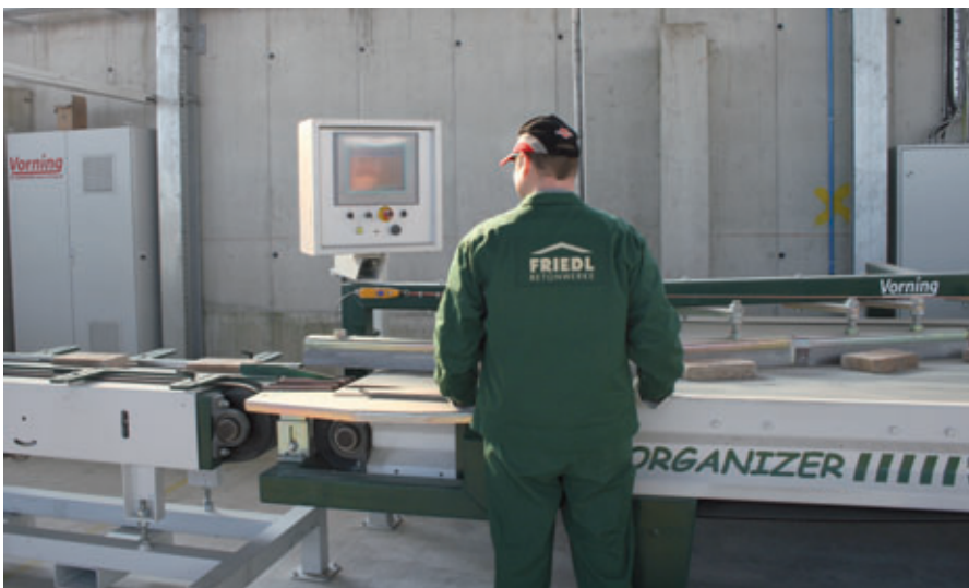
Only one employee – essentially in a monitoring function – is necessary for the complete ageing and packaging process
