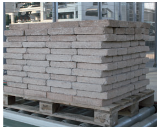
The finished packets of concrete blocks are transported via a roller conveyor to the outside area. A special technique allows the layers to be stacked offset from one another
