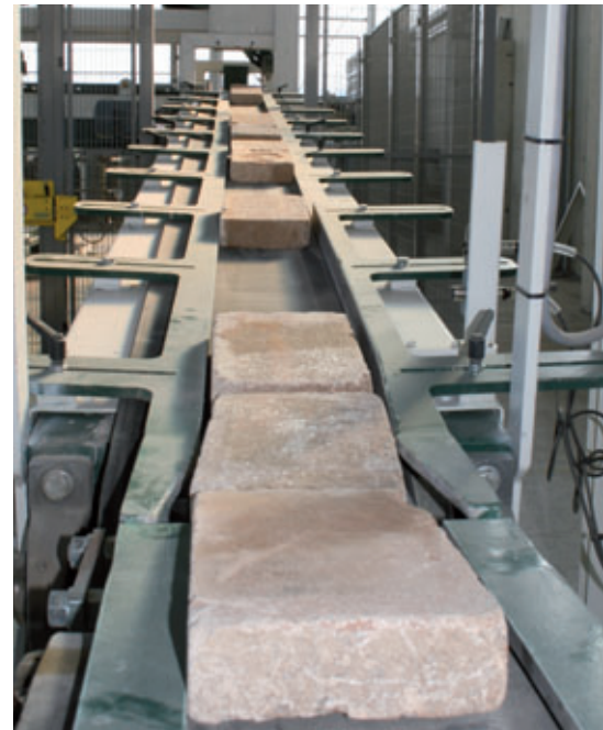
The sorted blocks are transferred by the Organizer onto the intermediate storage belt which constantly replenishes the supplies for the packaging unit
