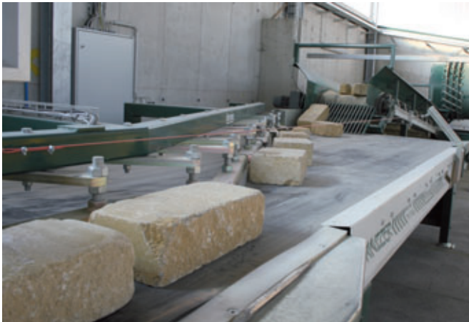
Large concrete blocks can also be aged and packaged in the plant
