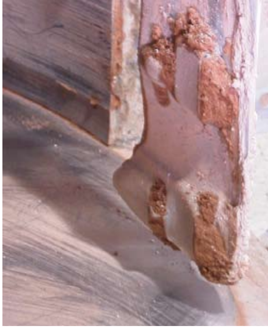
Fig. 2 Adherent materials in the mixer caused due to a worn bottom scraper. For removing this several times a day much time might be needed.
