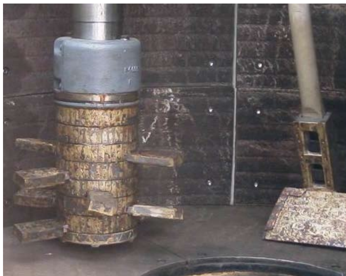
Fig. 1 High-performance mixer furnished with WIDIA-tipped mixing tools.
